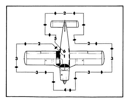
b. Insure that wings and control surfaces are free of snow, ice or frost.
